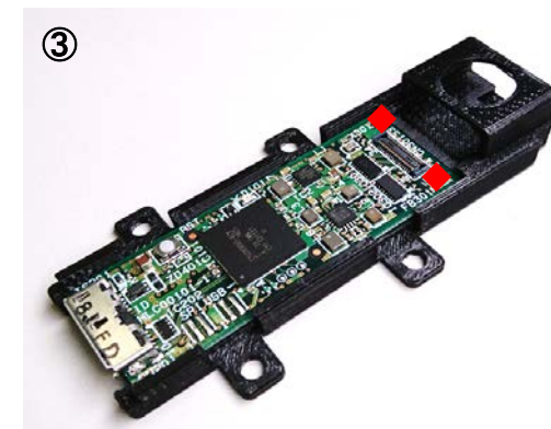
3. Push the mark of ♦ and insert the board into the case.
