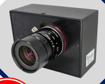
An event-based vision sensor is designed to emulate how the human eye senses light. The sensor detects the luminance changes in each pixel and extracts only those that exceed the preset threshold value then outputs the event "coordinate, polarity, and time". This operation is performed independently and asynchronously for each pixel.
